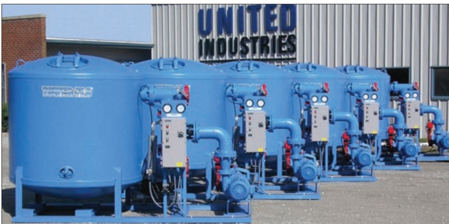
Five, TFB-66 Filter Systems, 475 gpm each, with backwash from static supply and backwash lockout by five
