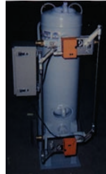
TFCL-12-Automatic-Portable-HITEMP filter system for 250°F water with "positive isolation" valve arrangement and custom control sequence with "cool down" cycle timer.
